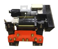
WB Wheel Brakes apply force generated by springs on both sides of crane wheels. Oversized brake shoes with bonded friction material apply on the side flanges of idler wheels, providing the friction forces, and thus, braking capacity.
