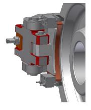
WB Wheel Brakes apply force generated by springs on both sides of crane wheels. Oversized brake shoes with bonded friction material apply on the side flanges of idler wheels, providing the friction forces, and thus, braking capacity.
