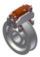
Designed as parking brakes to be applied when equipment comes to a full stop, WB wheel brakes can be also used as dynamic brakes in an emergency (e-stop). By applying spring force directly on the wheel flanges, they minimize the amount of stress and strain otherwise placed on sill beams and truck assemblies of a crane.
